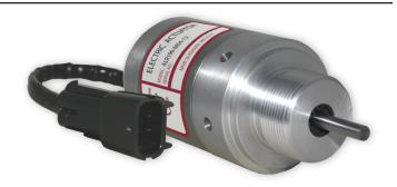
are not equal, the speed control unit changes the actuator current which alters the actuator's magnetic force. The actuator's output shaft position is proportional to the magnetic force generated and is counter-balanced by an internal return spring. The motion of the actuator shaft against the fuel rack of the engine causes a change in fuel delivery until the engine speed equals the speed control unit preset engine speed setting.
